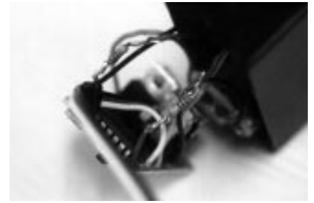
Figure 5. In this photo the two 2.2 k-ohm resistors have been soldered in place.
